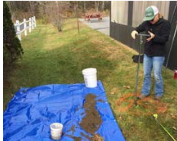
Figure B12. Soil testing was completed adjacent to the Wilkins Harley Davidson parking lot to confirm soil infiltration potential.
