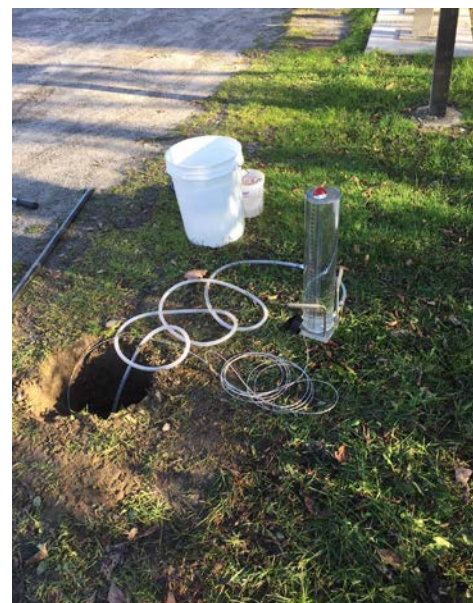
Figure B15. An example of the Constant-Head Borehole Permeameter Test in progress using a Johnson Meter.
