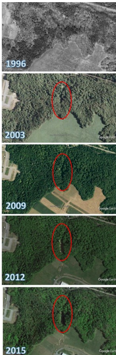
Figure B20. Progression of gully formation from 2003 to 2015.
