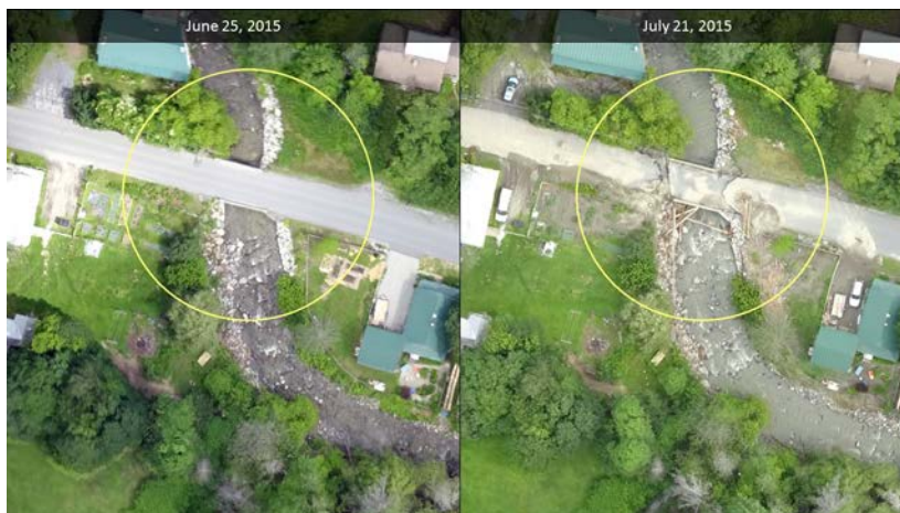
Figure C2. Flooding-related damage in Great Brook following a high intensity rain event. Imagery collected by the University of Vermont Spatial Analysis Lab (2015).
