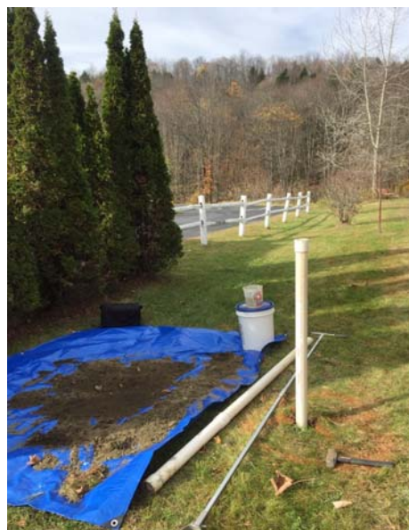
Figure B16. Infiltration testing using the falling head method in progress at the Wilkins Harley-Davidson site.
